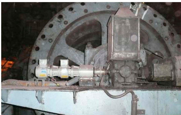
After: More precise signals because of robust combination of bearing block and heavy duty encoders.
