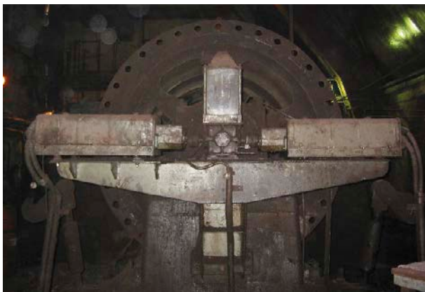
Before: Old skip-car control mechanism with two mechanical geared cam limit switches.
