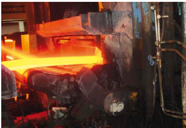
Loopers in hot rolling mills are working under extremely rough conditions.
