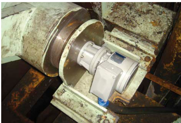
Looper encoder with heavy-duty ball bearings and special lubrication for long lifetime.
