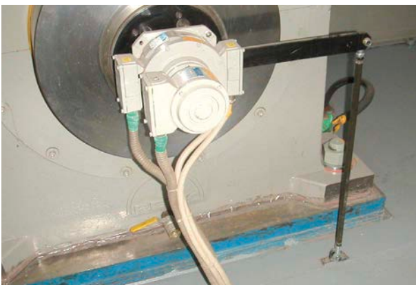
Electronic overspeed switch EGS 41 mounted on an incremental encoder FGH 6.
