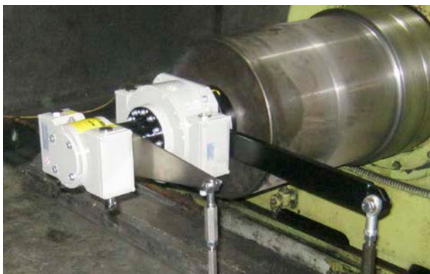
Turnkey encoder modernization by engineering support package with site measuring, construction, mounting and commissioning support.
