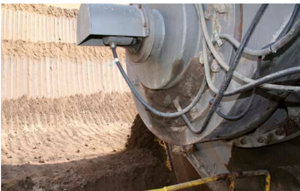
The high-resolution encoder FGH 40 detects even the smallest changes of rotation speed very rapidly.
