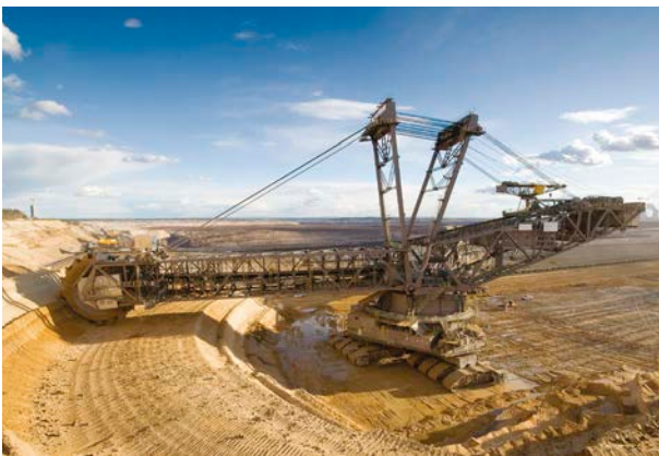
The operator cabin of the bucket wheel excavator is located at the end of the boom.
