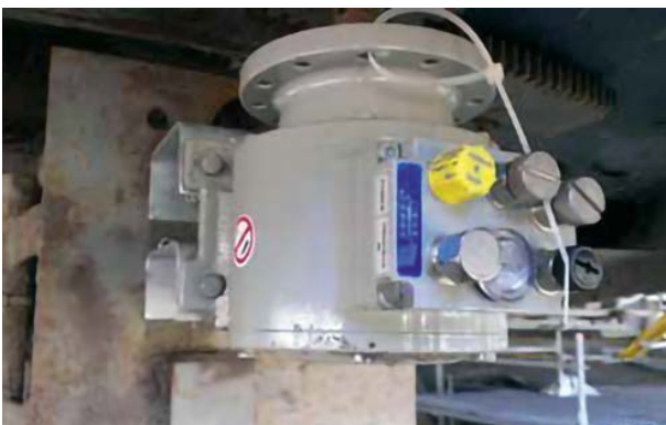
After: The safety certified absolute encoder AMPN 41 provides safe position actual values to the safety plc.
