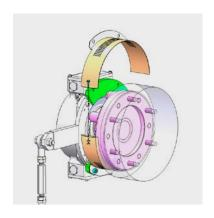
The two halves of the cover are each attached to the retaining plate and screwed together
