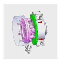
Mounting the retaining plate on the FGH 6 flange
