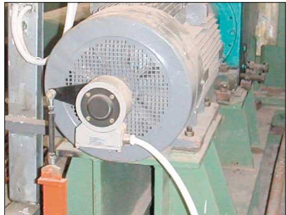
Hollow shaft encoder type FGH4K with screw-in type shaft, with torque bracket mounted to self-ventilated motor.
