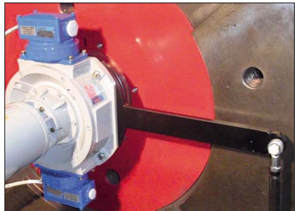
Hollow shaft encoder type FGH8EES with electronic over-speed switch, mounted on a big motor shaft, with lever arm – long version.
